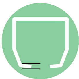
2-degree taper keeps the trolley centered
